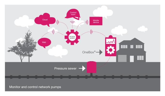
Imagine if you could monitor your pressure sewer units in real time and operate them remotely.
